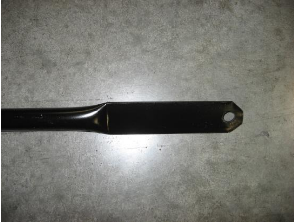
TANK BRACE- Long smash
