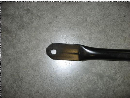
TANK BRACE- Short smash
